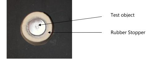
Then rubber stopper was inserted to the test jar cover. Two strips of 2.5 cm x 15 cm of test samples were attached with test jar cover. Please see below picture.
