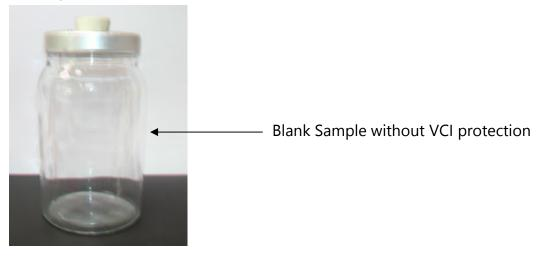
The four test sets were stored for a period of  $(20\pm0.5)$  hours at a room temperature. At the end of the storage period, the jar covers were removed from the test jars, the freshly
